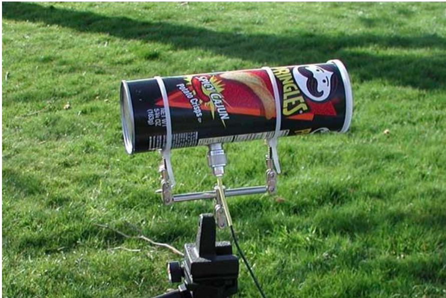
Pringles Antenna ( Spicy Cajun model required ) ~7 dBi gain
