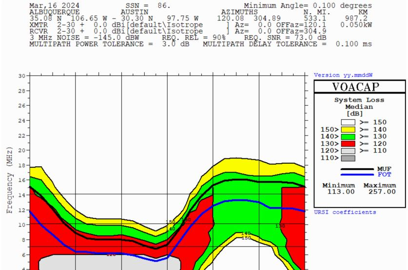
VOACAP is a prediction tool that predicts the signal path loss between the transmitter and the receiver.
