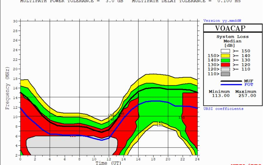
**Path Loss Example** Frequency = 14.131 MHz LOSS = 130.74 dB
