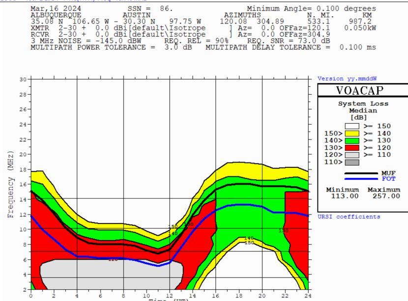
Path Loss defines how much a signal will be attenuated as it propagates from the transmitter to the receiver.
