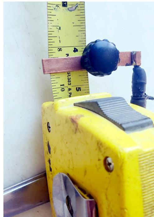
17. A small cleat is used to hold the paracord / string at the desired height, as needed. This makes life much easier, trust me. If your tape measure has a thumb lock, use it! OK, you're pretty much ready to go do some HF radio!
