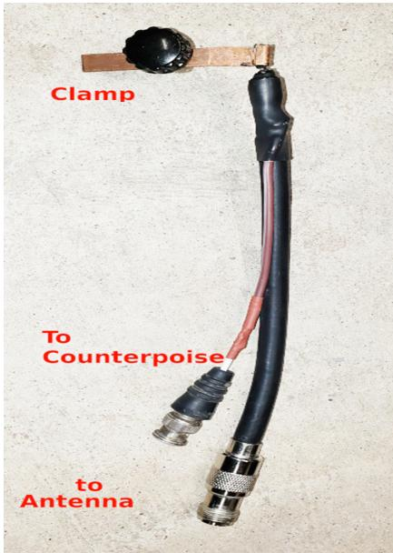
7. The antenna connection is a short piece of RG-8 COAX cable. The thick copper center will hold up to normal use. Keep it as short as possible to keep the SWR low.
