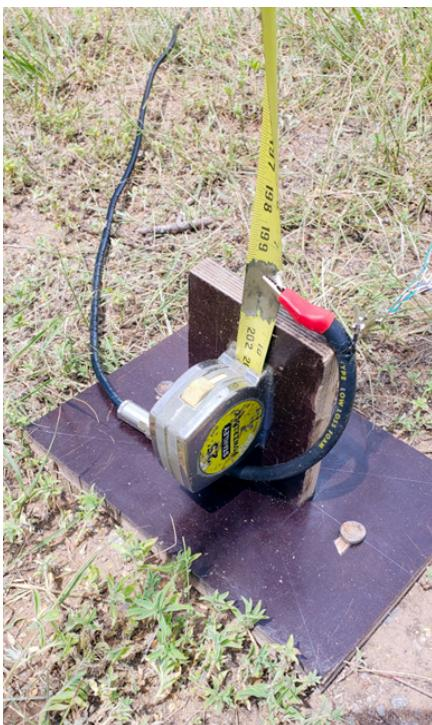
This antenna is great for QRP rigs or 100 Watts with no issues. How well you "clamp" to the bare steel portion of the tape measure is important. Do not let it move! I have made contacts with S-9 reports on both USA coasts, as well as Canada. This antenna works!
