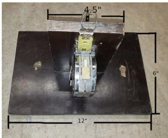
1. Make the base 6"x12". The vertical support for the tape measure should be 4½"x6". This gives you enough clearance around the tape measure.
