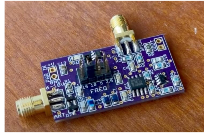
Grape PSWS receiver/mixer board 0.88 x 1.56 inches
