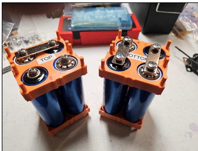
Figure 9: The Assembled Basic 4-cell LiFe Battery Unit with Labeling
