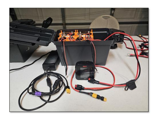
The ammo-can configuration also provides for easy drilling of holes, which should be protected with rubber grommets for cable feeds
